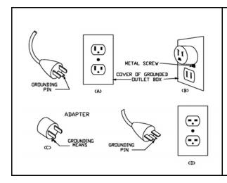
**WARNING**: This water cooler is for use on 120 volt outlets only. The cord has a plug as shown in A. An adapter as shown in C is available for connecting three-blade grounding-type plugs to two-slot receptacles. The grounding lug extending from the adapter must be connected to a permanent ground such as a properly grounded outlet box. The adapter should not be used if a three-slot grounded receptacle is available.
